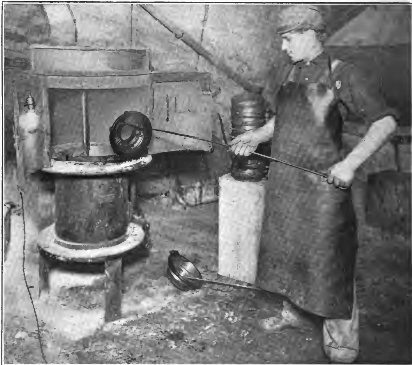
DEPICTING THE METHOD OF HEAT-TREATING STEEL TO BRING OUT KINETIC QUALITIES, USING SALTS OF METALS FOR THE BATH, AT WOOD'S PLANT
